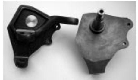
CB Performance forged 2in/51mm dropped spindles are available for both the king and linkpin suspensions (top) and ball-joint suspensions (above), and allow the fitment of high performance disc brakes.
