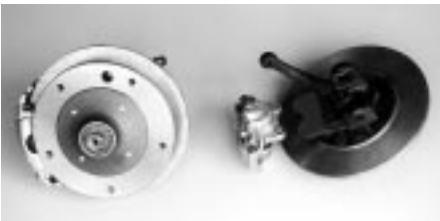
Autocavan supply a 11in/280mm disc brake kit (using Golf GTi calipers) for early and late Beetle suspension types. This design retains the early five-bolt wheel pattern. (Courtesy Autocavan).
