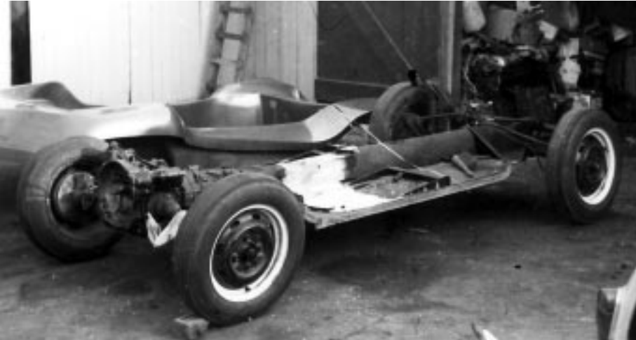
A Beetle chassis prepared to accept a dune buggy bodyshell. The simplicity and strength of the rolling chassis design has made it ideal for building buggies. (Courtesy John Jackson).
