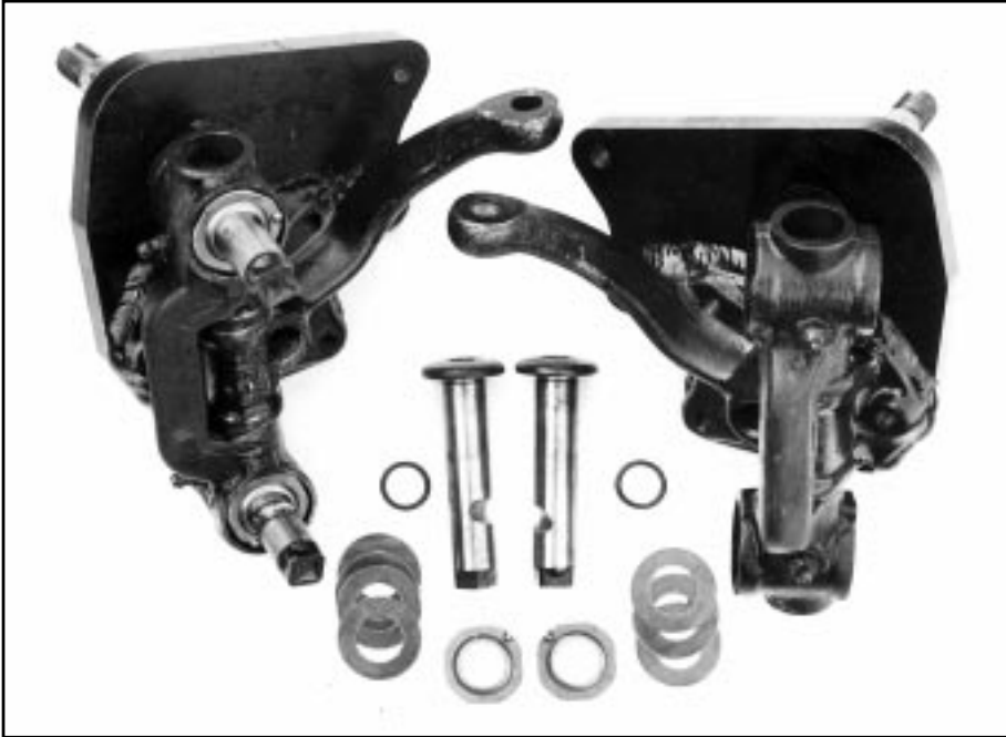
Linkpins use shims to set the correct suspension geometry. This JaTech setup allows the use of disc brakes, and lowers the suspension by 2 inches (51mm).
