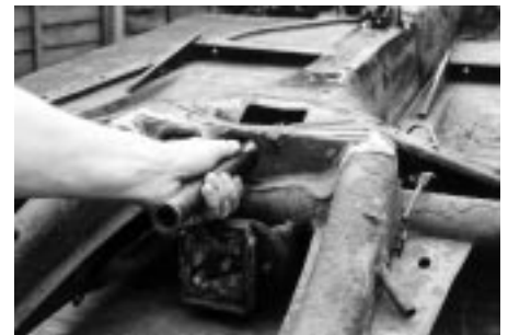
With the gearbox and gear-shifter removed, the selector rod can be physically pushed from its resting place in the plastic support bush with a long rod inserted through the rear section of the chassis.
