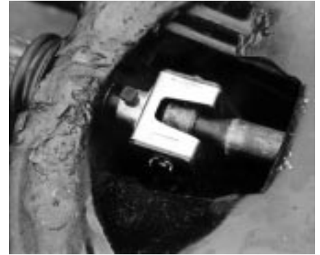
The rear access plate is removed to allow the gearbox 'hockey stick' selector to be disengaged from the long gear selector rod which runs within the chassis backbone.
