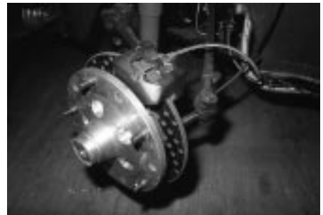
This cross-drilled disc brake set up (for early Beetle suspension) from Neal, features race-quality Wilwood calipers and lightweight billet aluminium hubs.
